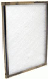
Typical size = 20" X 25" X 1" Low air resistance and good for poorly designed systems having undersized ductwork. **These filters only remove the larger dust particles (big chunks).** Use these filters during the air conditioning season when maximum air flow is needed. Maintenance: Replace every two to three months max.
